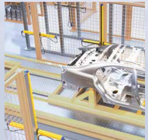
2. PRESENCE DETECTION BEHIND A LIGHT CURTAIN FOR HAZARDOUS AREA PROTECTION
