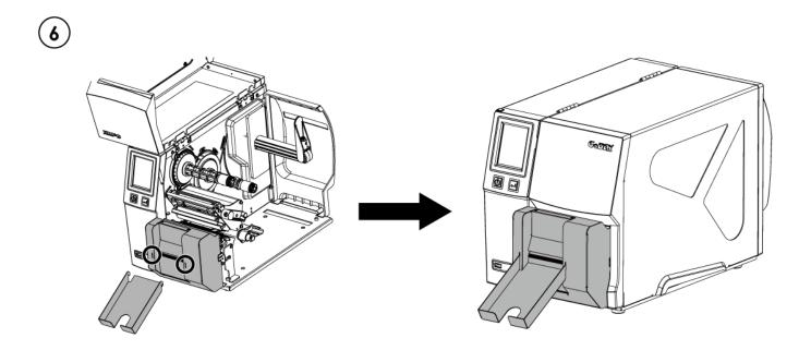
$1. \hspace{0.5cm} \textbf{Snap the ticket tray to the cover of cutter to complete the installation}. \\$
