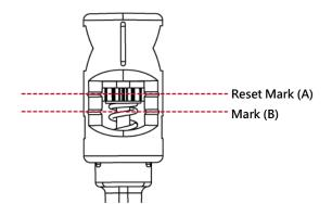
Turning the screw left increases the pressure, while turning it right reduces the pressure.
