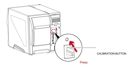
Press C-button for 2 seconds, it will make an auto-sensing to calibrate the label and ribbon's parameters.
