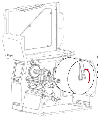
Place the label roll on the label supply hub, pushing it right up to the printer housing.
