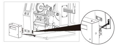
3. Plug in the cable connector to the bottom5-PIN jack of printer's left panel
