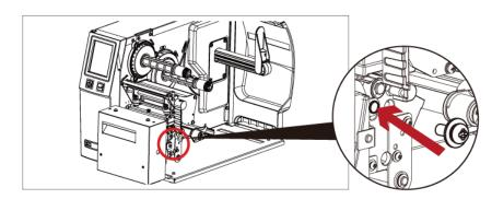
5. Hold the perforation cutter module firmly and tighten the screw
