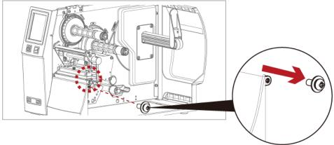
2. Remove the cover panel by pushing to the direction of right-hand side.
