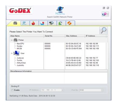
Click the magnifier icon to search the Godex printers which are connected via Ethernet port in you network environment. Once a connected Godex printer is detected, it will be listed on the start page.
