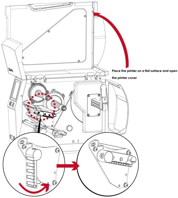
Turn it anticlockwise to a top right position as shown in the illustration
