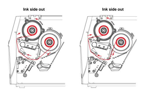
Pass the ribbon under the print head and back up on the other side. Attach it to the empty ribbon core.
