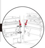
4. Insert the perforation cutter module to dock with the printer
