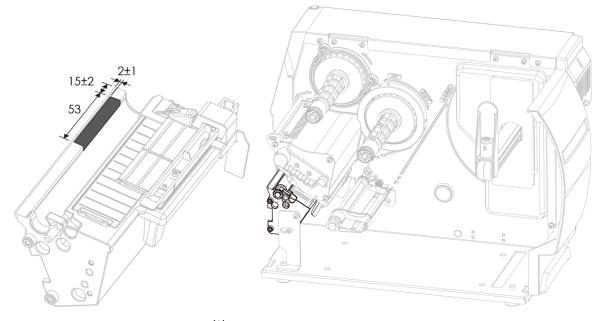
XPaste position of Anti-Static tape
