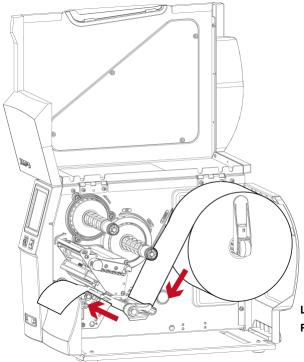
Load the label roll into the printer as shown in the illustration. Pass it through the printer as indicated by the red arrows.
