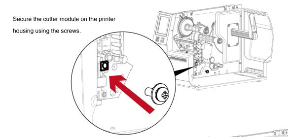
Finish the cutter module installed.
