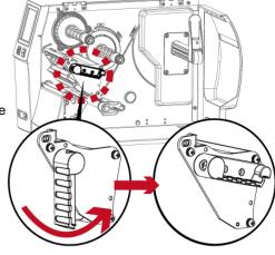
Hold the print head module, pull out the TPH cable smoothly.
