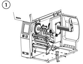
1. Assemble the Platen module bracket.
