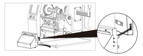
4. Insert the cutter module to dock with the printer
