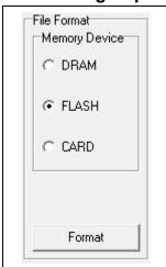
This feature is used to delete all the files for the specified memory device.
