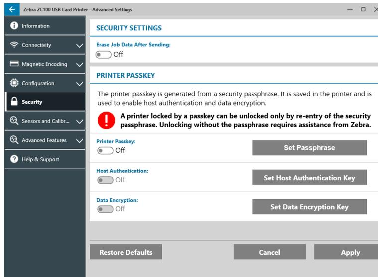
In the **Security Settings** section, the user can set Erase Job Data After Sending On or Off. This will prevent the last print job from being recovered.
