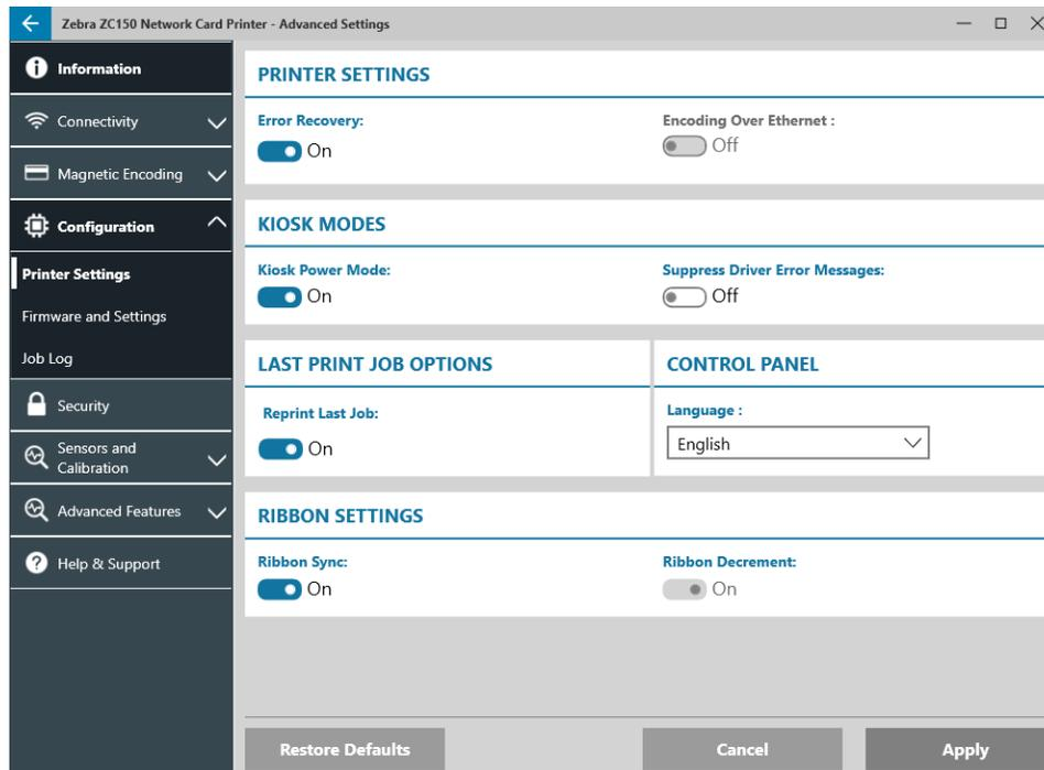
In the **Printer Settings** section, the user can turn Error Recovery on or off and Encoding over Ethernet on or off.
