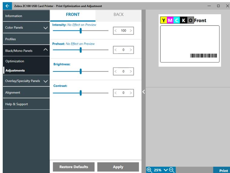
The **Intensity** adjustments gives the user control over how dark or light the black/mono panel is printed.
