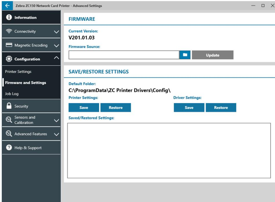
In the **Firmware** section, the user is shown the current firmware version, and can update to the latest firmware.
