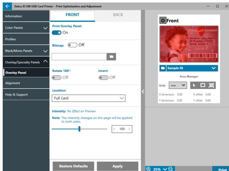
**Print Overlay Panel** On/Off determines if the panel is used. If the selection is set to On, the overlay panel is used and the remaining options are available; if the selection is set to Off, printing of the overlay panel is skipped.
