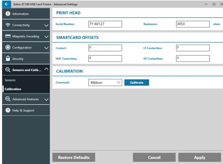
The **Printhead** section tracks the serial number and resistance value of the currently installed printhead. Use this section when installing a new printhead to enter new values.
