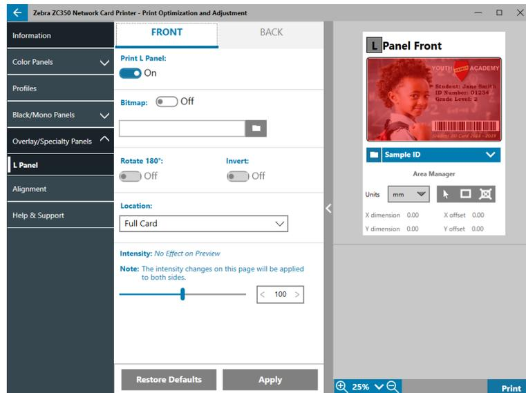
The options for the L panel are the same as for the Overlay panel. When both L panels are printed on the same side of the card, and the bitmap option is enabled, the bitmap is only printed using one of the L panels. This allows security features to be printed while maintaining a protective overlay.
