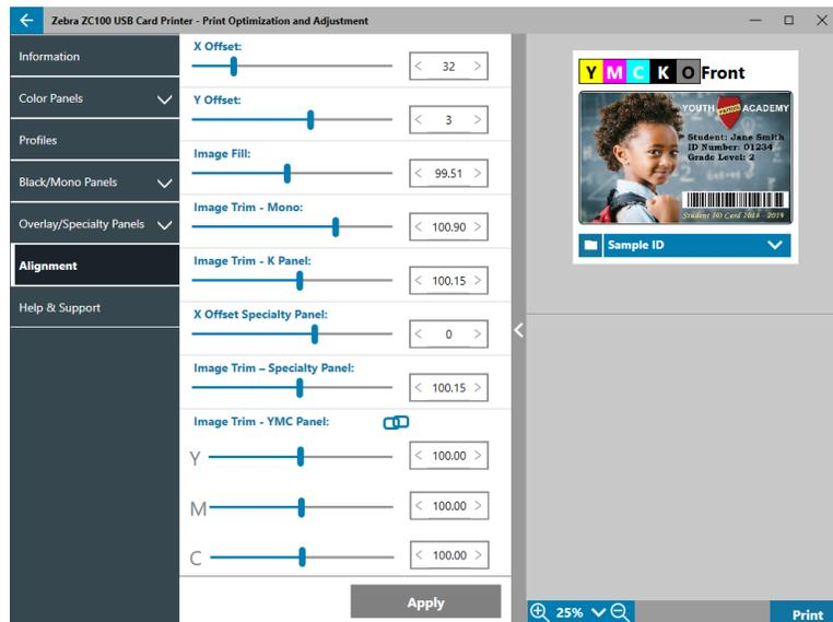
**X Offset** adjusts the placement of the image along the long axis.
