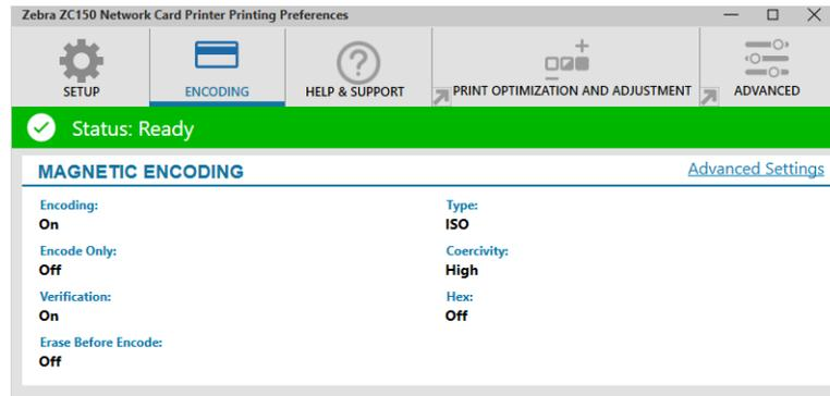
**Encoding** – When set to On, a card with a magnetic stripe will be encoded when a print job with magnetic encoding data is sent to the printer. When set to Off, the printer will not encode any cards.
