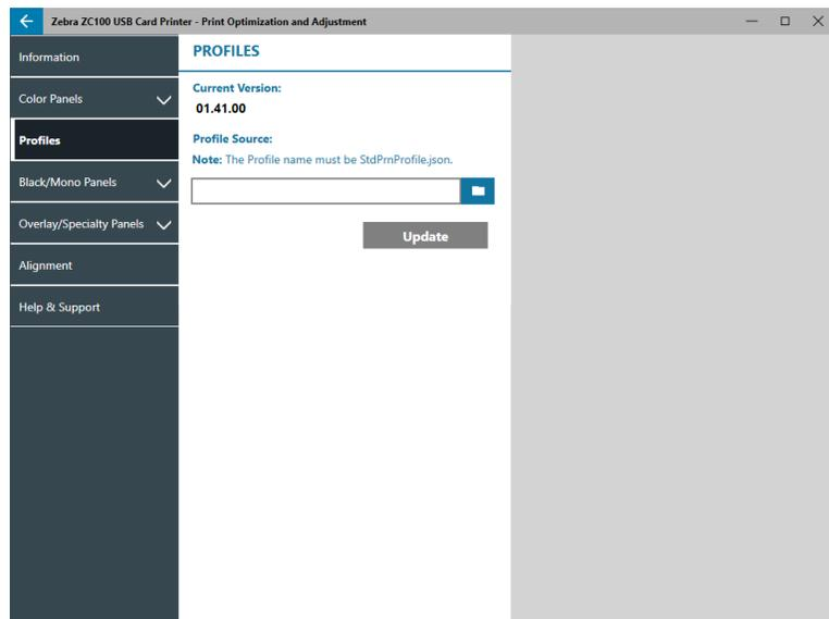
The **Profiles** page is used to load a different profile to the printer. The profile is used to control many functions of the printer, such as print tensions, amount of energy used for different panels, etc.
