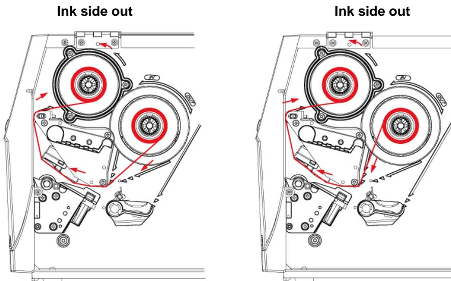
Pass the ribbon under the print head and back up on the other side.
