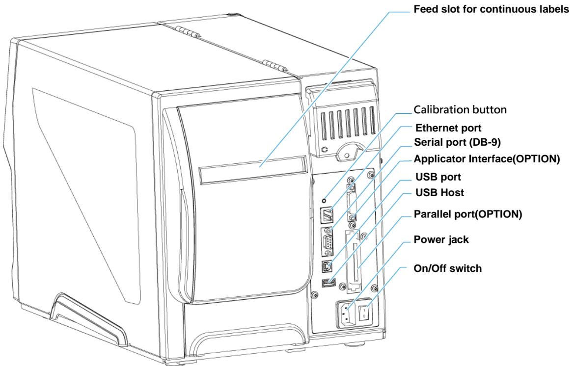
•The Internal View of Printer
