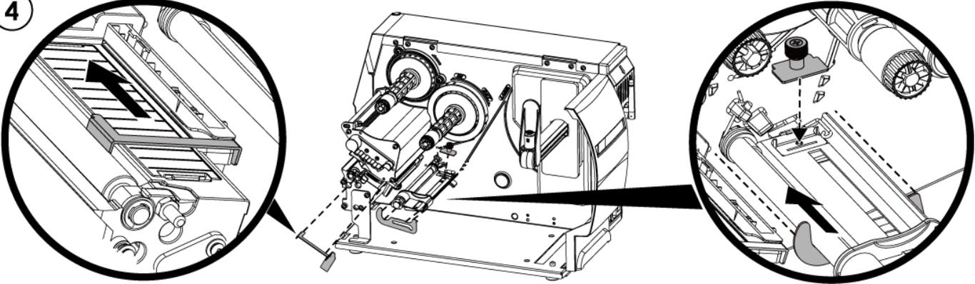
1. Install the label bracket and the label holders respectively. During the installation, push the parts to the left end and fix them with double-sided tape.
