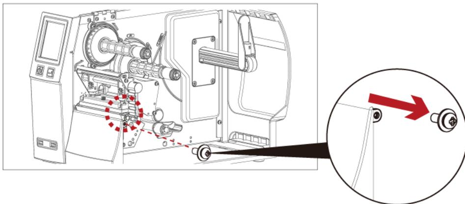
2. Remove the cover panel by pushing to the direction of right-hand side.
