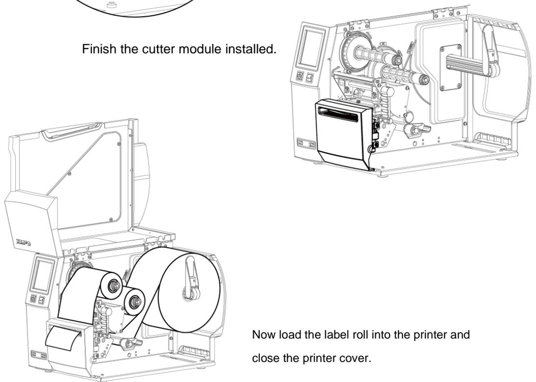
Now load the label roll into the printer and close the printer cover.
