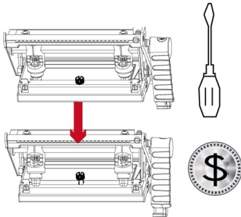
using a screwdriver or a coin to loosen the screw
