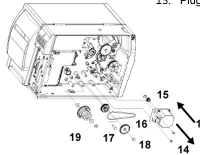
14. Remove the motor combination
