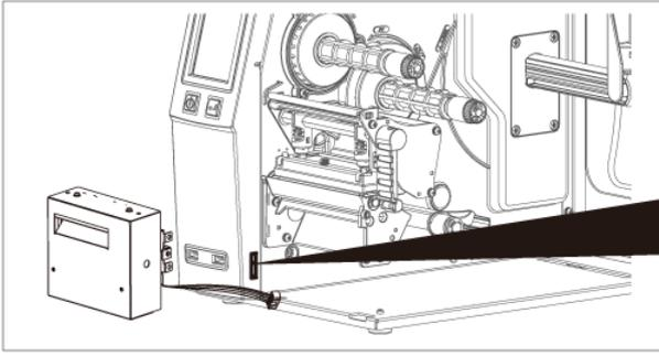
3. Plug in the cable connector to the bottom 5-PIN jack of printer's left panel
