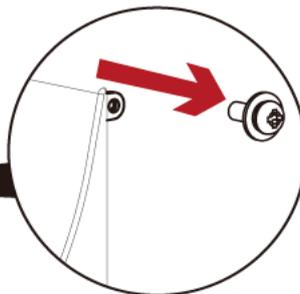
2. Remove the cover panel by pushing to the direction of right-hand side.
