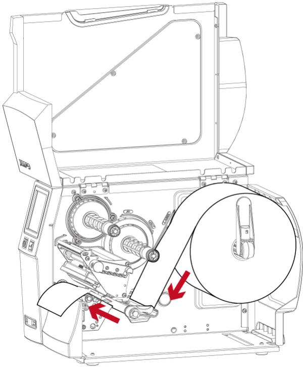
Load the label roll into the printer as shown in the illustration. Pass it through the printer as indicated by the red arrows.
