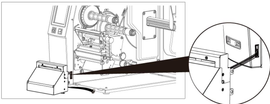
4. Insert the cutter module to dock with the printer
