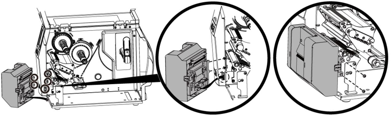
1. When installing the cutter, plug in the cable into the socket first, then insert the left side of the cutter into the mechanism fillister.(as shown in the picture)
