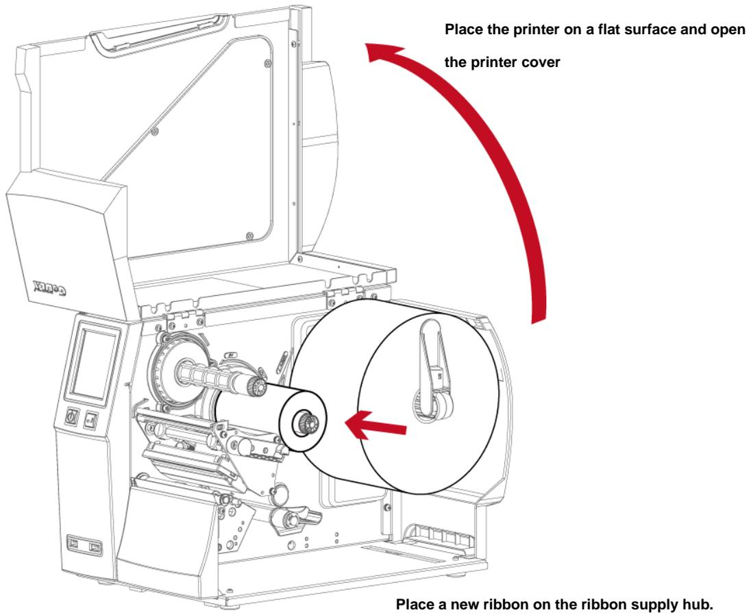
The two illustrations as below show you how to install the ribbon depending on the ribbon type (ink side in or out).
