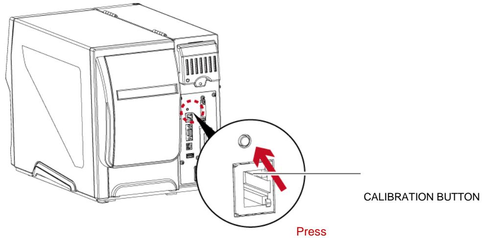
Press C-button for 2 seconds, it will make an auto-sensing to calibrate the label and ribbon's parameters.
