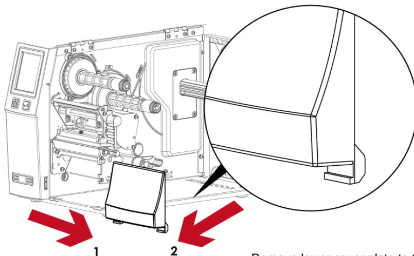
Remove lower cover plate to the a little bit right then can get out.
