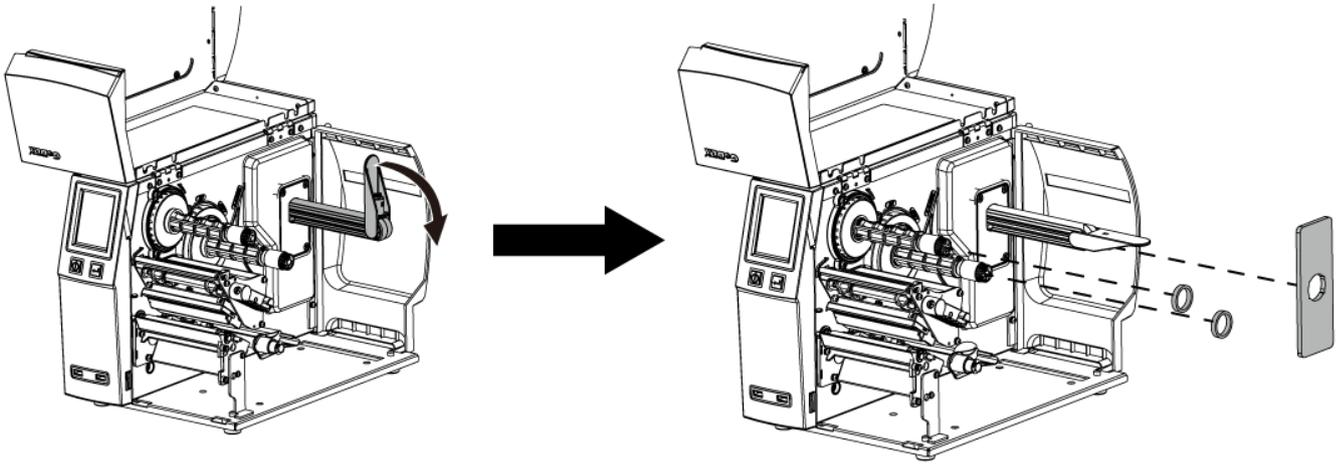
1. Assemble the label stop plate and plastic tubes.
