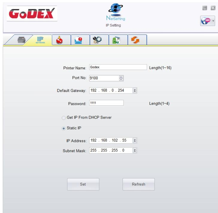
The screenshot shows the 'IP Setting' window in the GoDEX NetSetting software. The window title is 'GoDEX NetSetting IP Setting'. The interface includes a toolbar with icons for printer, IP, and other settings. The main area contains the following fields and options:
