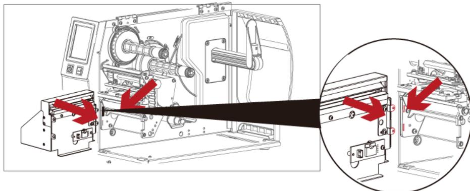
5. Hold the cutter module firmly and tighten the screw
