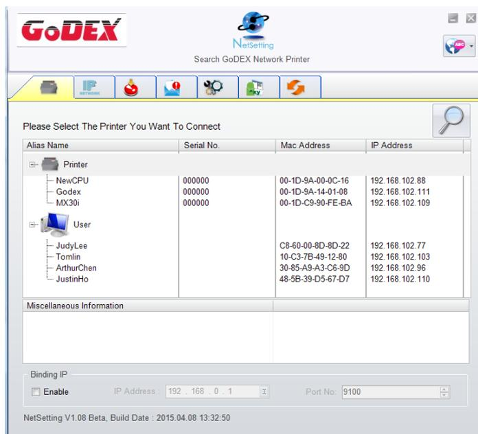
Click the magnifier icon to search the Godex printers which are connected via Ethernet port in your network environment. Once a connected Godex printer is detected, it will be listed on the start page.
