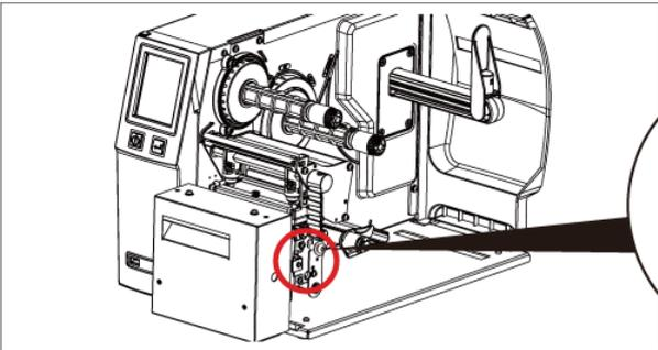
5. Hold the perforation cutter module firmly and tighten the screw
