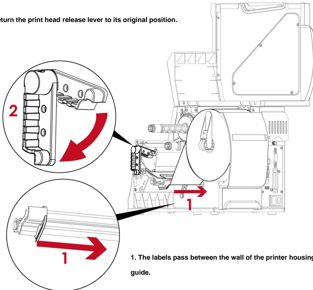
1. The labels pass between the wall of the printer housing and the adjustable paper guide.
