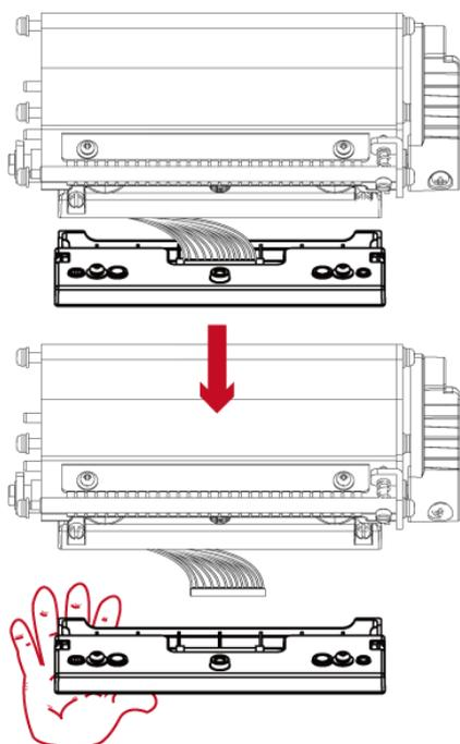
Hold the print head module, pull out the TPH
