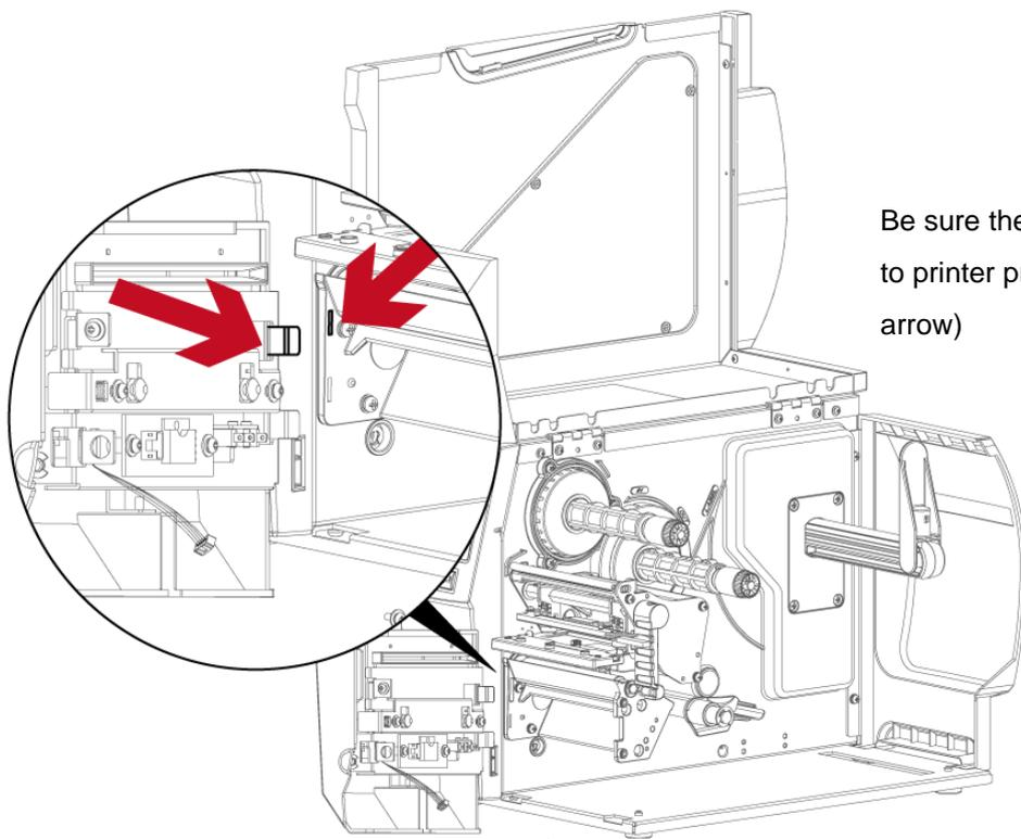
Be sure the cutter module insert to printer properly. (see red arrow)
