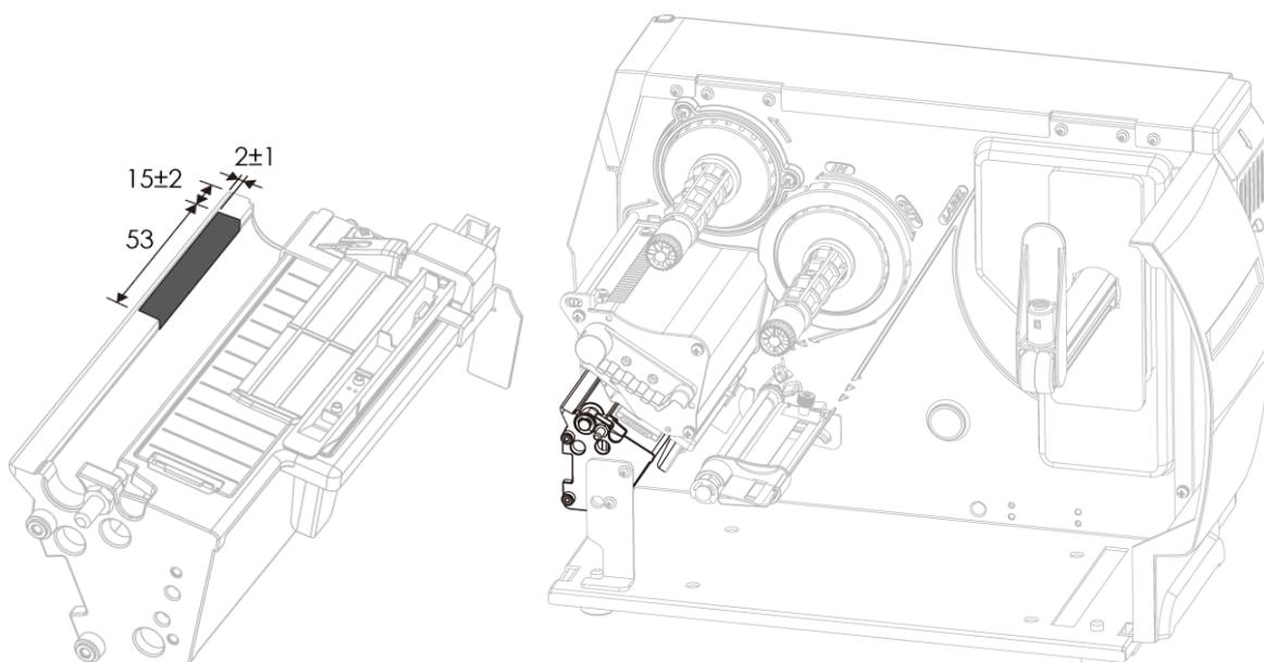
※Paste position of Anti-Static tape
