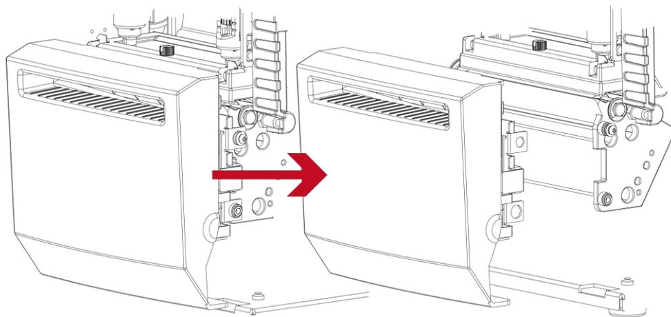
Switch off the printer before removing the CUTTER.
