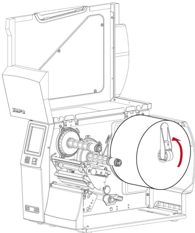
Place the label roll on the label supply hub, pushing it right up to the printer housing. (Do not apply too much pressure to avoid damaging the label stock.)
