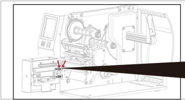
4. Insert the perforation cutter module to dock with the printer
