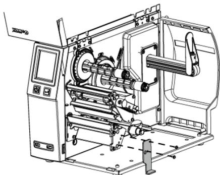
1. Assemble the Platen module bracket.
