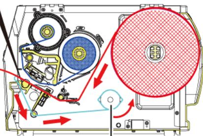
3. Pull the Liner back to rewinder shaft and rotate it in 2~3 circles
