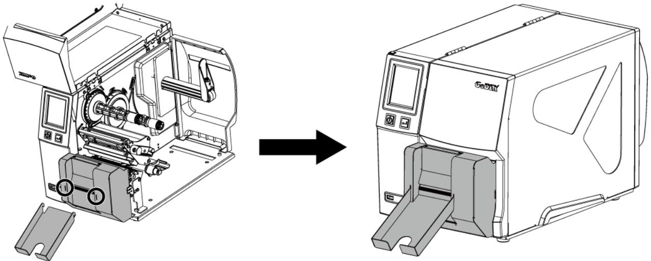
1. Snap the ticket tray to the cover of cutter to complete the installation.
