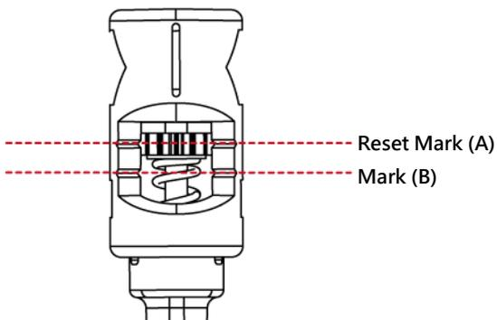
Turning the screw left increases the pressure, while turning it right reduces the pressure. Be sure not to turn the screw so that it goes below Mark(B).
