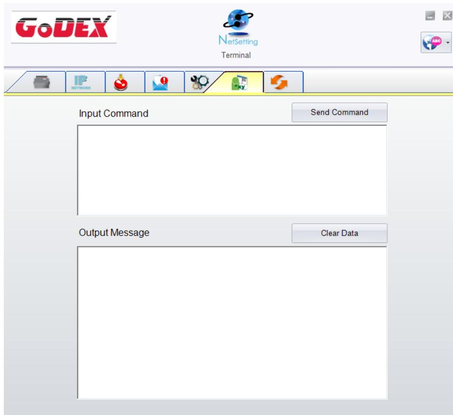
You can press "Send Command" button to send printer commands via Ethernet port and control the printer remotely.
