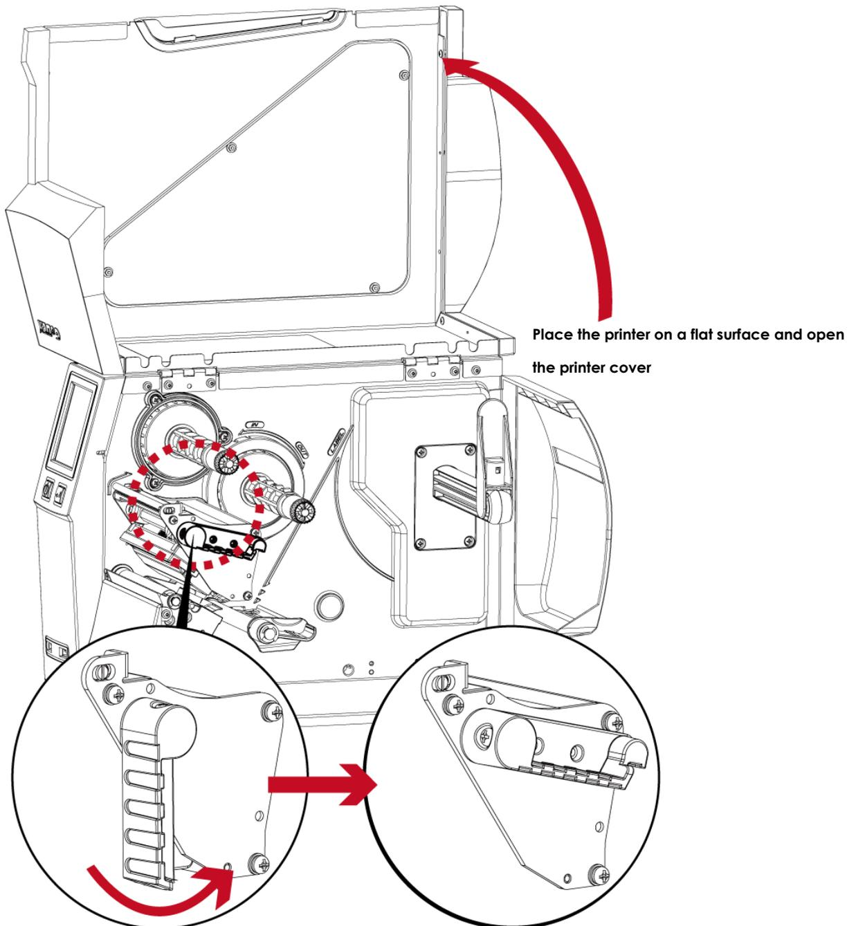
Place the printer on a flat surface and open the printer cover
