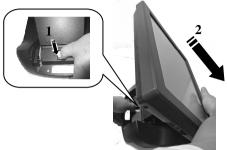
4. When the display goes down to a degree, loose the basefolding lever, as shown in the direction as indicated by the arrow below.
