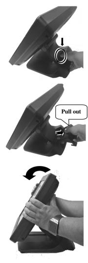
4. Determine that the terminal is tilted to the end, as shown in the right figure.
