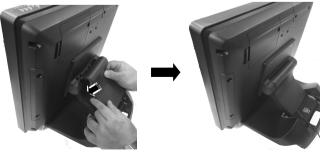
16. Shield the I/O cable exposure area with the cable cover.
