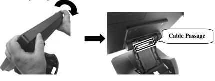
8. Make the connector, which will be connected to the I/O port of the terminal, pass through the cable passage of base stand.
